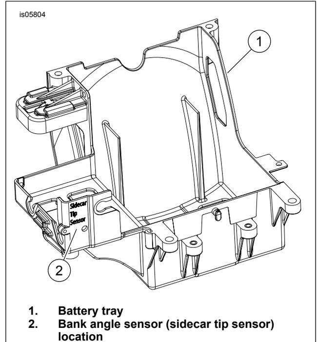
**Figure 1. Battery Tray for Bank Angle Sensor**
