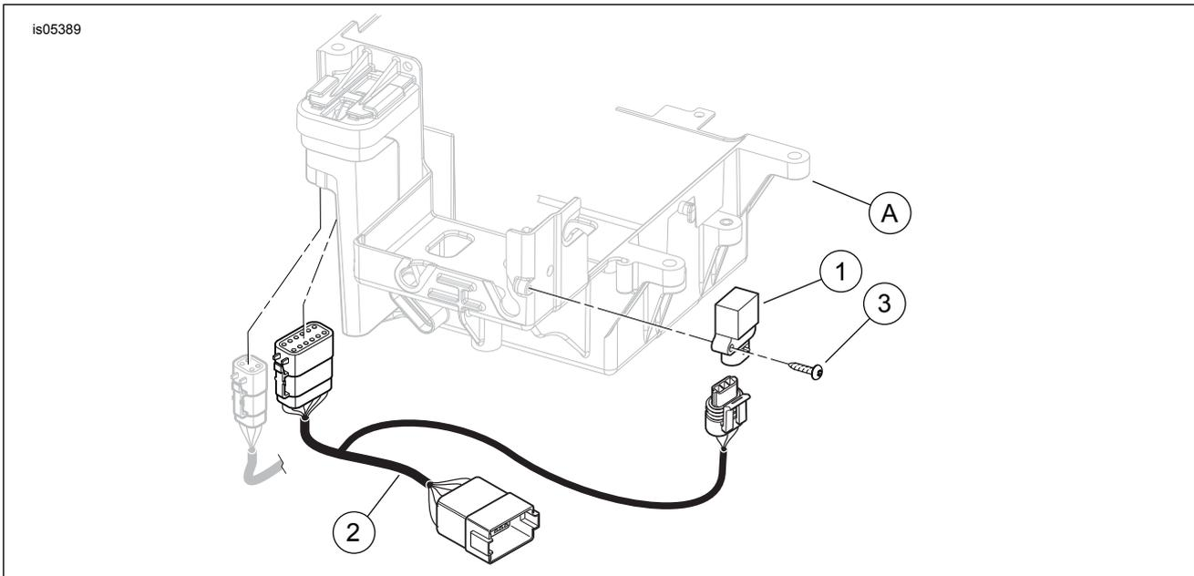
Figure 2. Service Parts, Bank Angle Sensor Switch Kit
