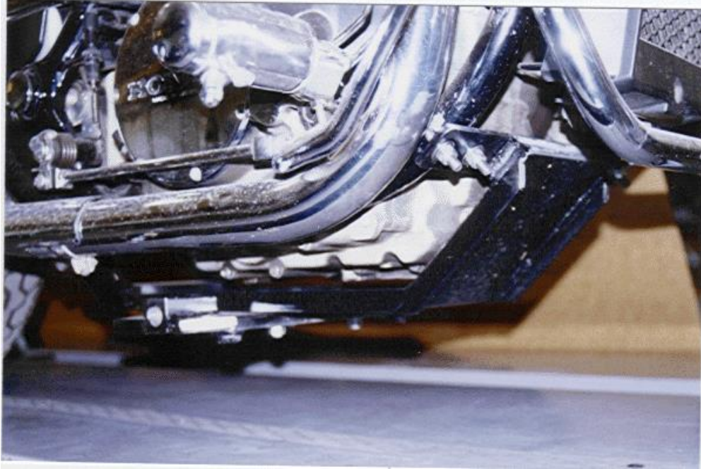
RIGHT SIDE BELLY BRACKET INSTALLED
