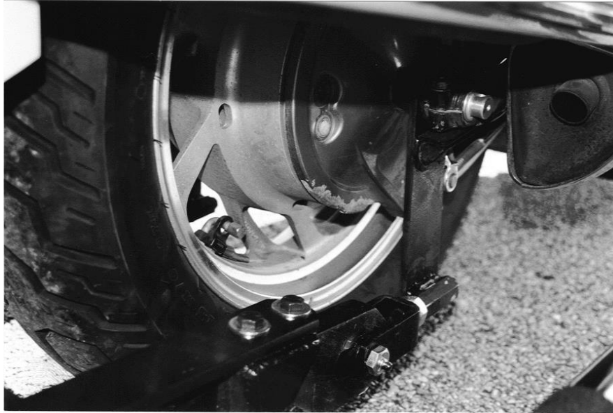
RIGHT REAR AXLE BRACKET INSTALLED
