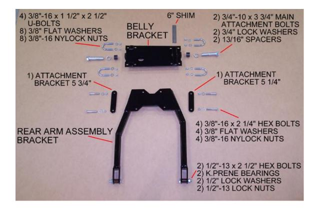
After installing the mounting hardware and attaching the Voyager frame to the belly bracket you may need a shim to make the motorcycle stand straight up and down.
