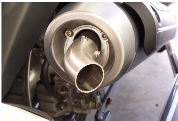
Exhaust tip installed on motorcycle.
