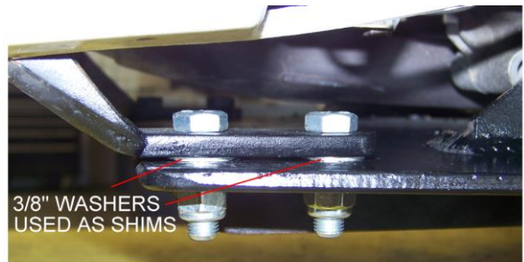
ILLUSTRATION OF SHIM PLACEMENT BRACKET PICTURED MAY NOT MATCH YOUR BRACKET
