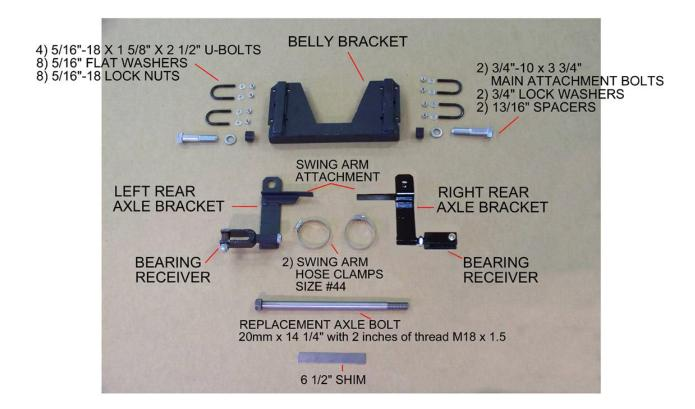
After installing the mounting hardware and attaching the Voyager frame to the belly bracket you may need a shim to make the motorcycle stand straight up and down.
